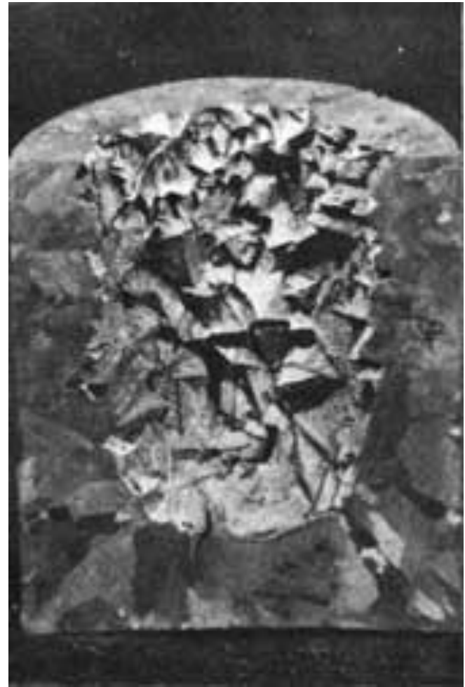
Crystal growth in gun metal casting dumped before solidification was complete.
