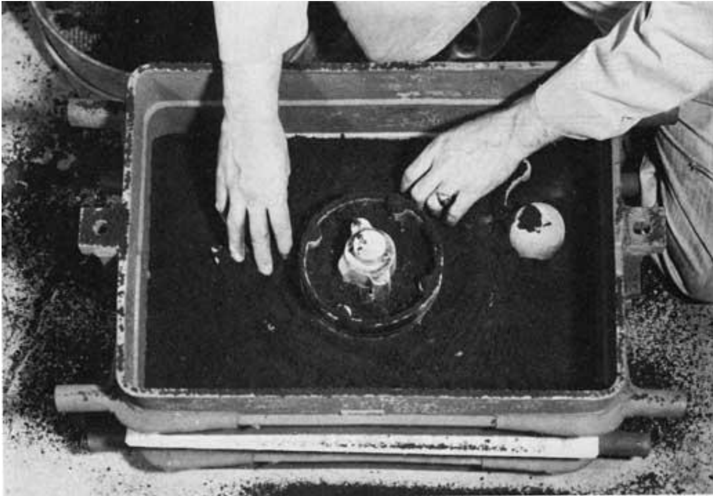
Hand packing riddled sand around the pattern.
