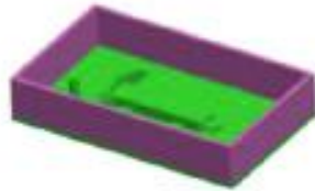
Place flask over cope portion of the pattern
