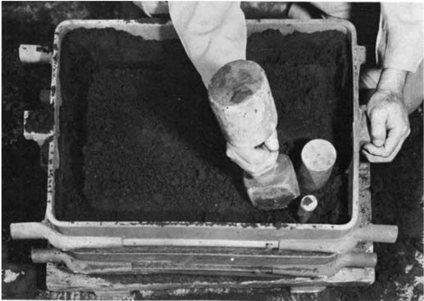
Ramming the partially filled cope.
