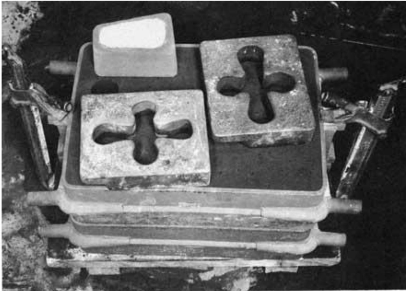
Clamped mold with weights and pouring basin
