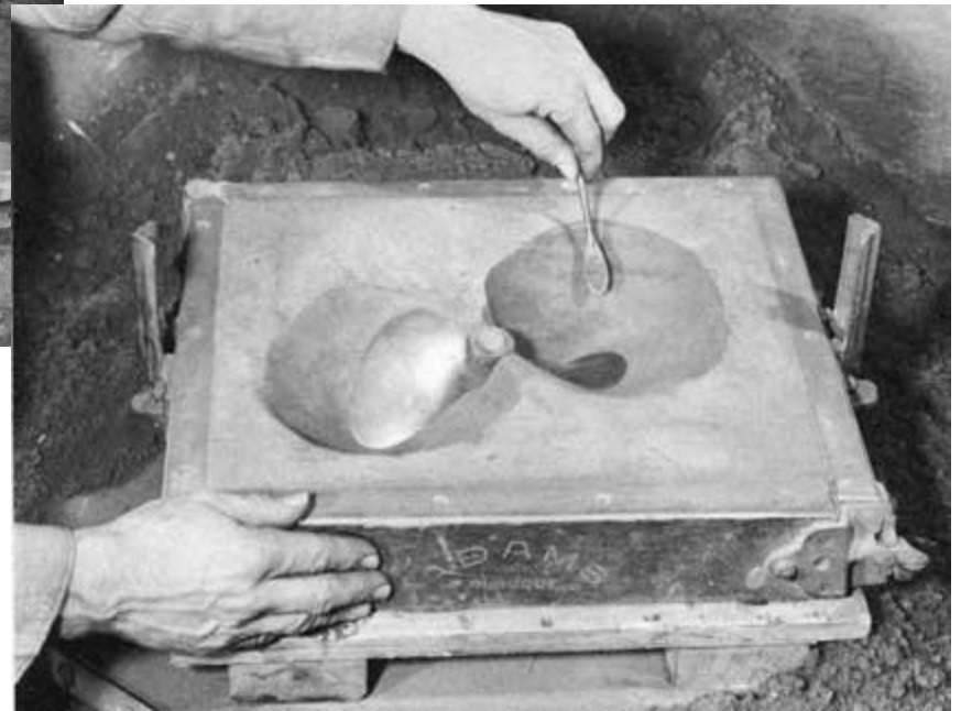
Propeller in the drag with parting line cut.
