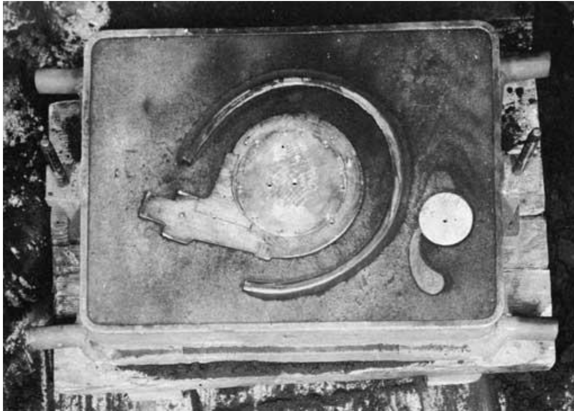
Drag ready for the cope.
