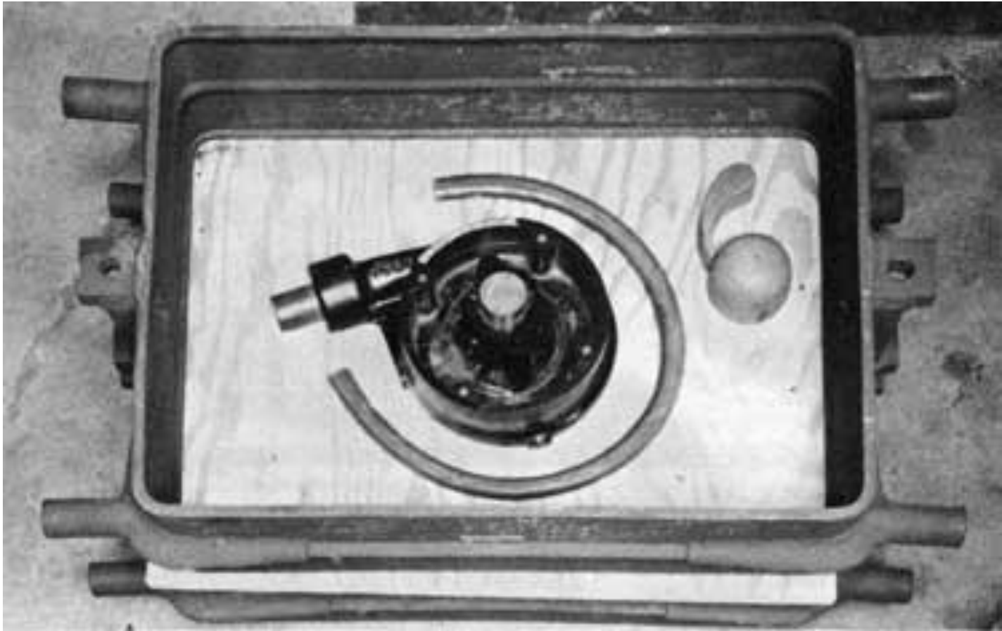
Pattern set in drag with gating system parts
