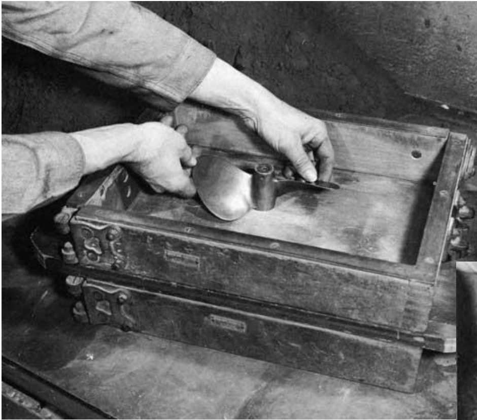
Propeller set in the drag.
